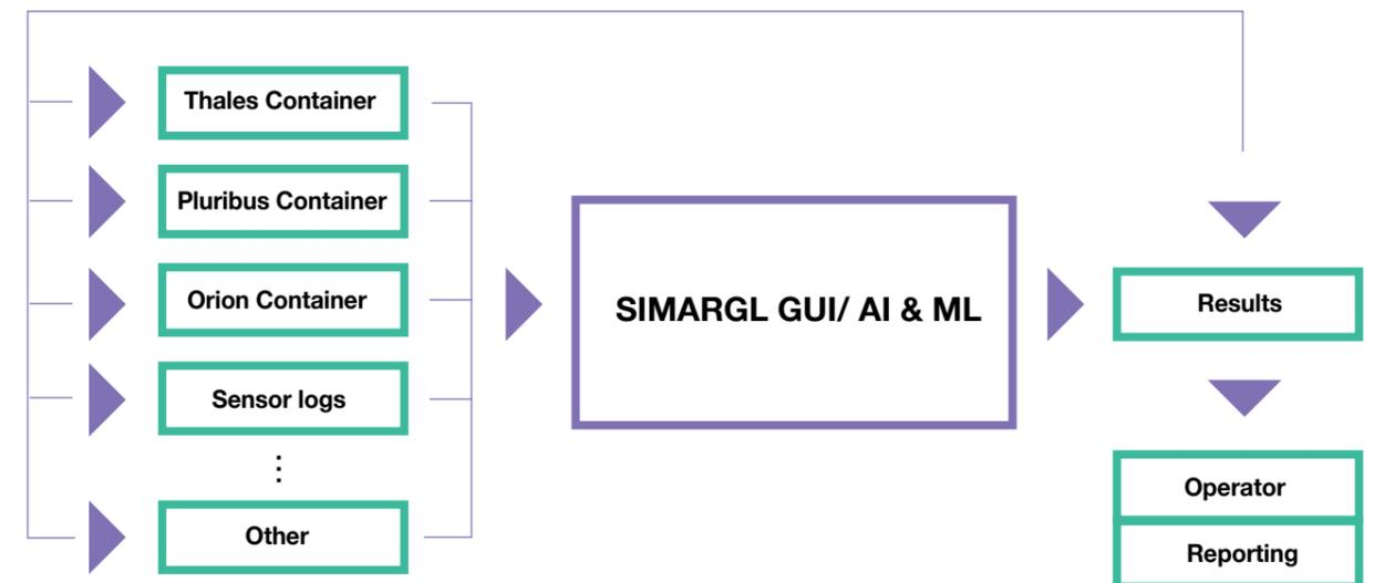
Schematic presentation of the use of case tests depending on the tools used in SIMARGL (Punch Platform by Thales, Orion Malware by Airbus Cybersecurity, Attack Prophecy and AISafe DNS by Pluribus One and BDE Engine by the Polish company ITTI).
