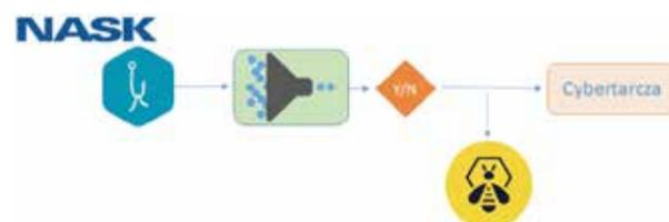
In the case of this mechanism, malicious content received through the established application interface goes to SOAR and are automatically blocked on CyberTarcza. The entire process from receiving the information to blocking at the network level took less than three minutes! Time not obtainable with manual approach.
